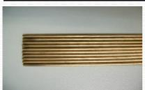
Recommended for surfacing applications which requires great hardness and high tensile strength. This alloy is commonly used for joining brass alloys and cast iron to carbon steel.
