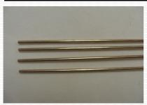
Recommended for Inert gas arc welding of copper, copper-silicon and copper-zinc base metals to themselves and to steel. Excellent for plain or galvanized steel sheet metal or other coated steel. Also used for surfacing areas subjected to corrosion.
